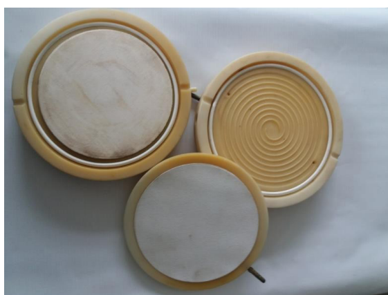
Figure 3. Membrane module of the installation
