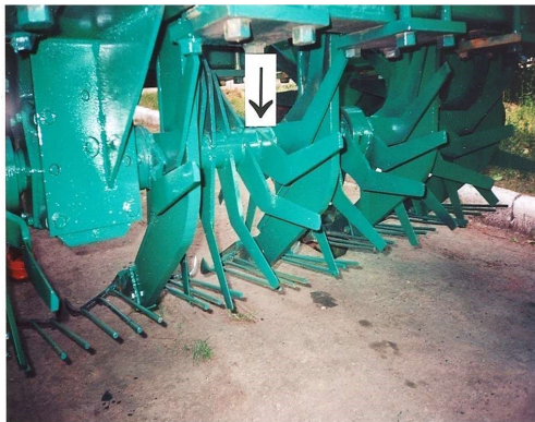
Figure 2. The rotor of an experimental tillage installation
